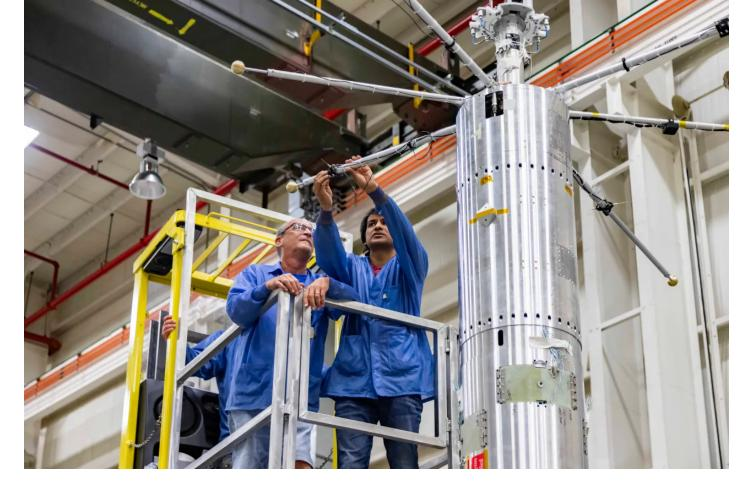
Mechanical technician John Peterson of NASA's Wallops Flight Facility and Barjatya check the six booms carrying the sensitive science sensors after a successful spin deployment testing. Credit: NASA's Wallops Flight Facility/Berit Bland
